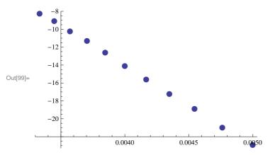
Now that we' ve linearized the data, we can do a much easier *linear* curve-fit using Mathematica's linear fitting routine, Fit. We're looking for the constant coefficient (which will be  $\frac{\Delta S}{R} + \log \left[\frac{k_b}{h}\right]$ ) and the linear coefficient (which will be  $-\frac{\Delta H}{R}$ ).
